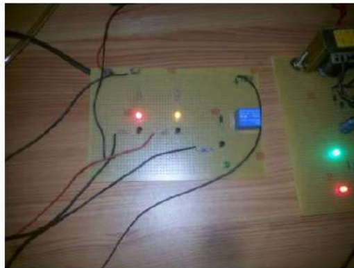
Figure 6: Yellow LED- Level 2 reached Indicating the tank is Half filled
