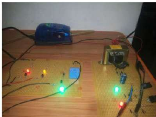
Figure 7: Green LED- Level 3 reached Indicating the tank is Completely filled
